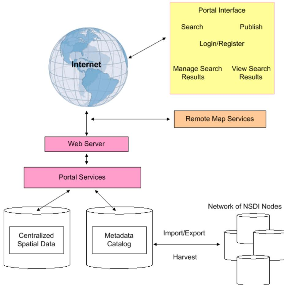
**Figure 4. System Components of the Central ASDI Portal**
